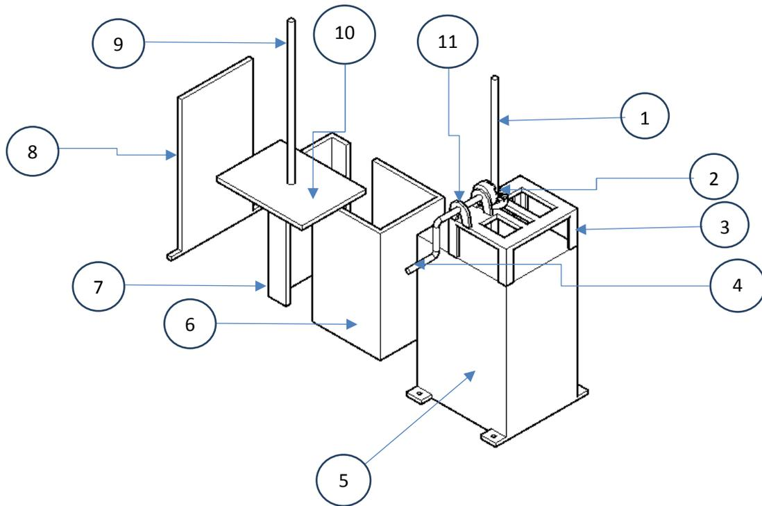
*Fig.2 Exploded view of the waste compacting device*
