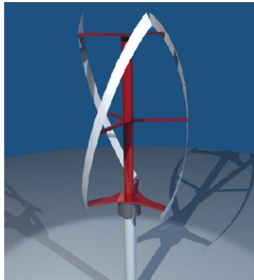
Fig. No. 07: Helical Blade Vertical-Axis Wind Turbine<sup>[19]</sup>
