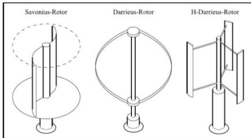
Figure No. 02: Main types of vertical axis wind turbines <sup>[20]</sup>
