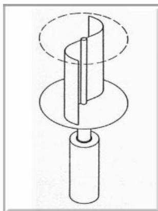
Fig. No. 08: Savonius type Vertical-Axis Wind Turbine <sup>[32]</sup>
