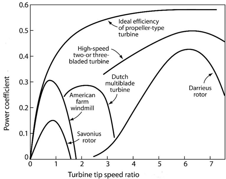
Figure No. 03: Power coefficient of different VAWTs [22]
