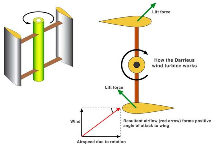
Fig. No. 05: Darrieus wind turbine operating principle<sup>[21]</sup>
