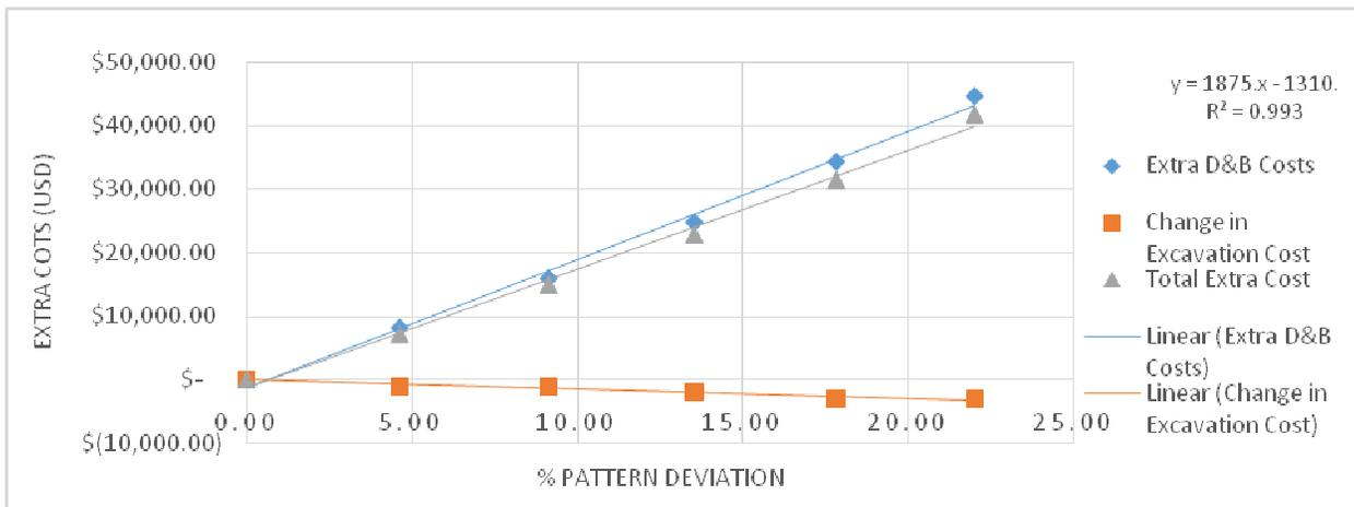
Figure 3: Total extra cost, extra D&B cost and Reduction in excavation cost against % pattern deviation for scenario 3
