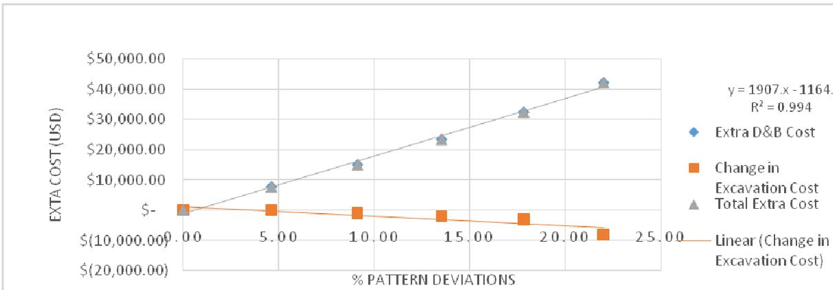
Figure .5: Total extra cost, extra D&B cost and Reduction in excavation cost against % pattern deviation for Scenario 5
