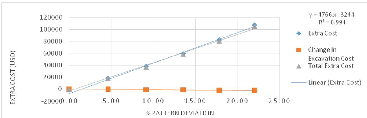
Figure 4: Total extra cost, extra D&B cost and Reduction in excavation cost against % pattern deviation for scenario 4
