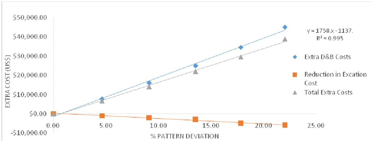
**Figure 1: Total extra cost, extra D&B cost and Reduction in excavation cost against % pattern deviation for Scenario 1**
