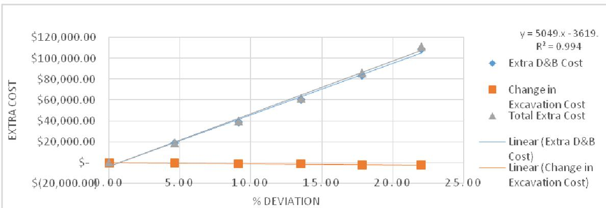
Figure 6: Total extra cost, extra D&B cost and Reduction in excavation cost against % pattern deviation for Scenario 6
