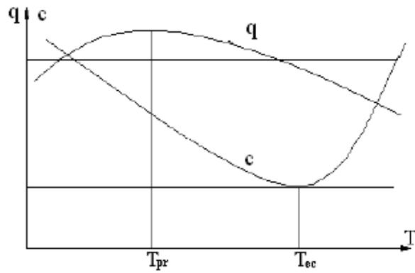
Fig. 2 Productivity  $q$  and cost  $c$  charts function of tool durability  $T$
