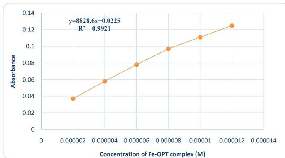
Fig. 2. Calibration curve for Fe-orthophenanthroline (Fe-OPT) complex.
