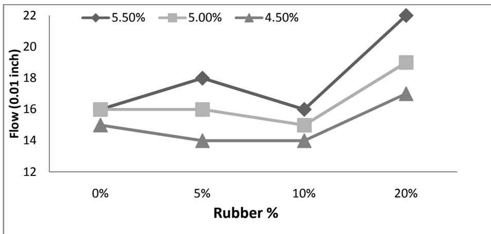
Figure (2): Relation between flow and rubber at different bitumen percentage
