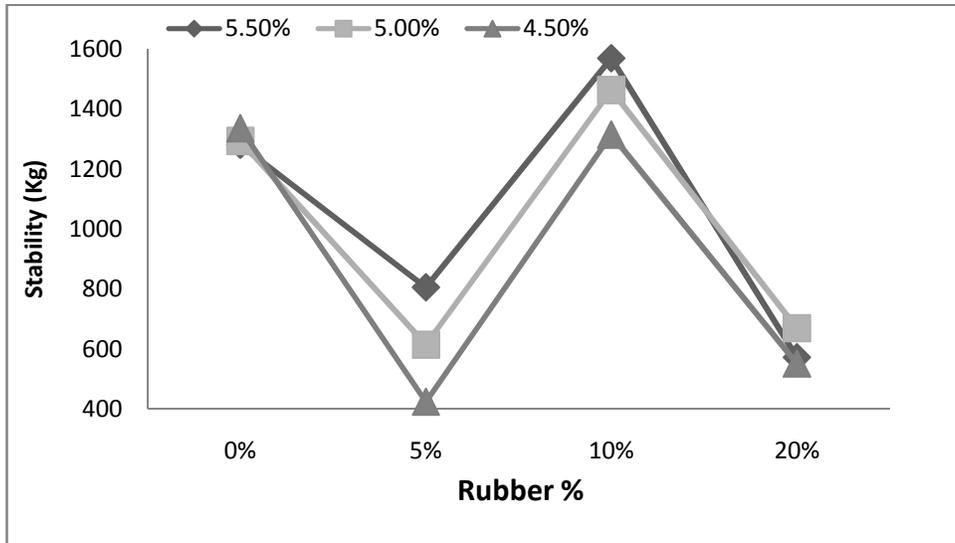
Figure (1): Relation between stability and rubber at different bitumen percentage
