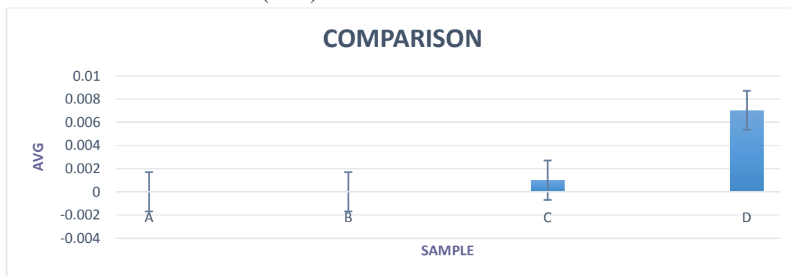
Figure 3.5 graph representing the average concentration of lead element in the samples. The error bars represent \pm SD
